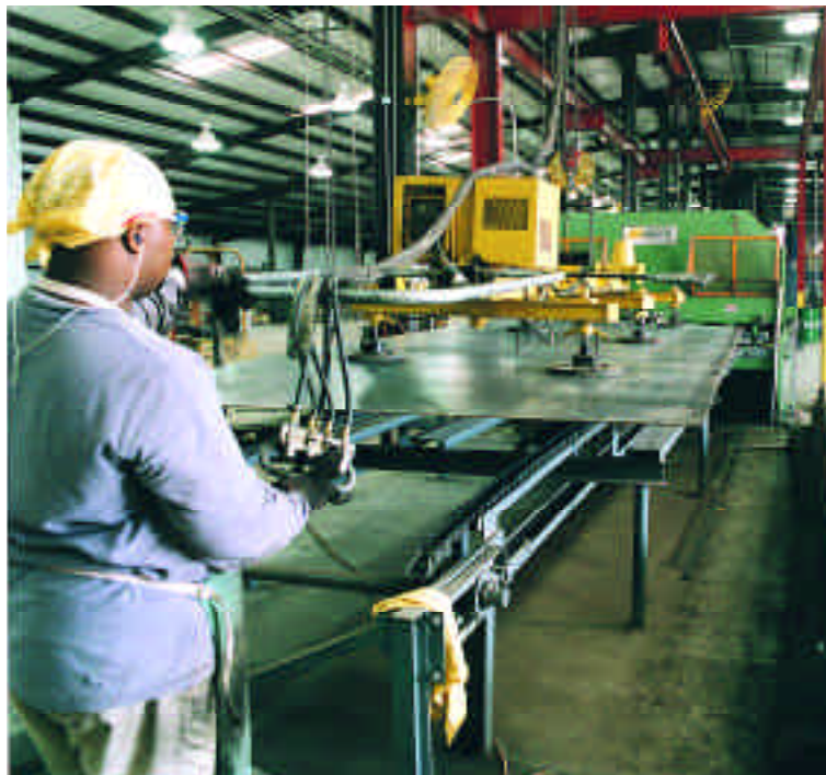
In the first manufacturing phase at Quality Steel’s plant, sheets of steel, brought in from Alabama mills, are sheared in half to be formed into two tanks. They then are rolled into a steel shell and tacked together.
