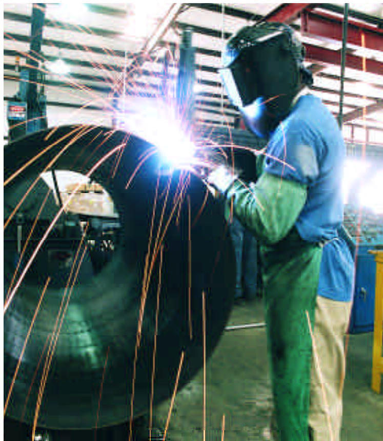
Once sheet steel is rolled into a cylinder, veteran welders at Quality Steel’s plant weld-tack seams together.
